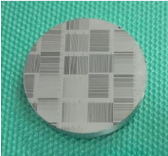
Figure 5. Chromium-masked DLC-coated SKD 11 before etching
