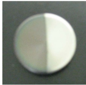
Fig. 4: DLC-coated SKD 11 sample after plasma ashing.
