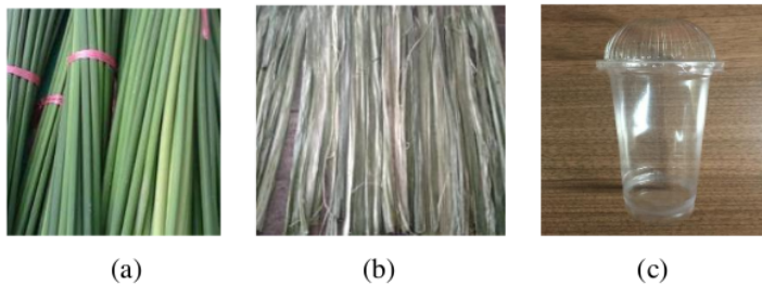
Gambar 4.1 Bahan komposit (a) Batang tanaman rumput payung (b) Serat batang tanaman rumput payung (c) Polypropylene (PP)
