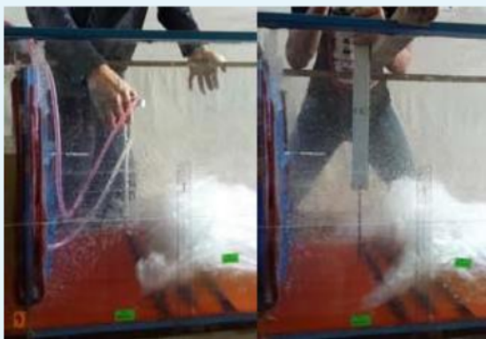
Fig. 2 : Water depth and velocity measurement for 12 section
