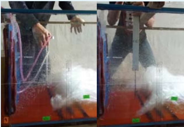
Fig. 2 : Water depth and velocity measurement for 12 section
