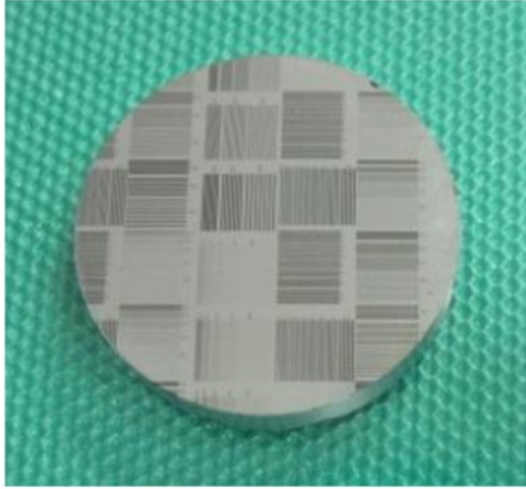
Figure 5. Chromium-masked DLC-coated SKD 11 before etching
