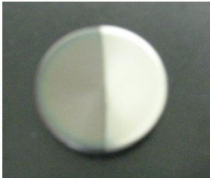
Figure 6 DLC-coated SKD 11 sample after plasma ashing
