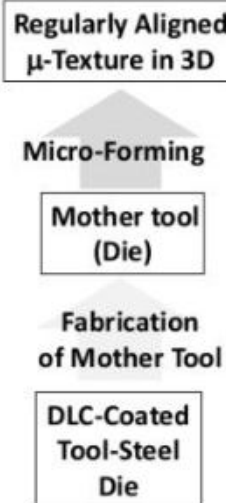
Fig. 1: Microforming procedure to fabricate the micro-textured aluminum sheet in mass-production.
