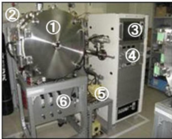
Fig. 2: High density oxygen plasma etching system to make micro-printing the designed micro-texture onto DLC-coatings. 1: Vacuum chamber, 2: RF-generator, 3: Control panel, 4: RF- and DC-power supplies, 5: Evacuation units, and,6: Carrier gas supply.
