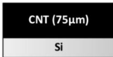
Fig. 6: CNT-coated silicon substrate before metallic masking.
