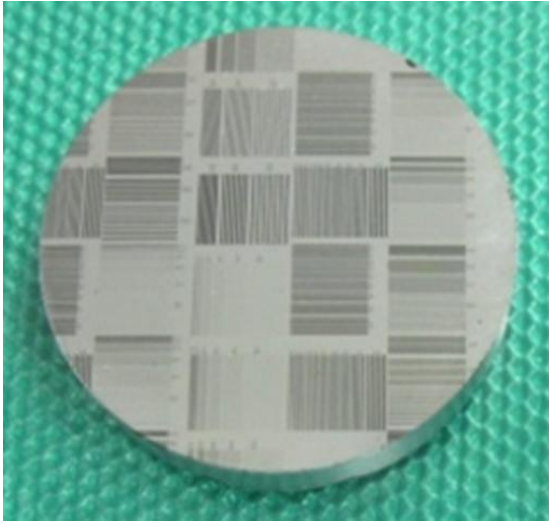
Fig. 5 Chromium masked SKD-11 specimen with variety of micro-groove pattern in the masking.
