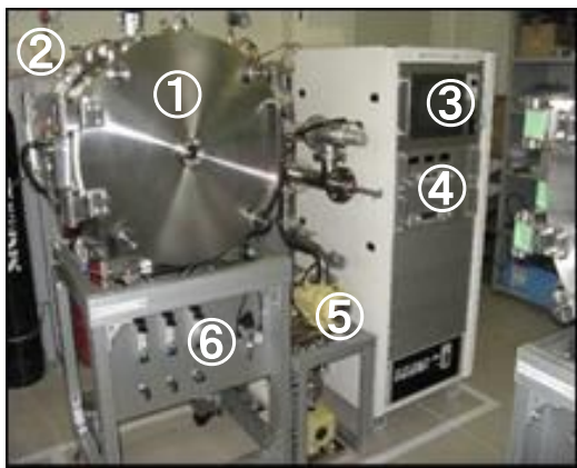
Fig.1: High density plasma etching system. 1: Chamber, 2: RF-plasma generator, 3: Control-panel, 4: Electric sources, 5: Evacuation system, 6: Gas supply.
