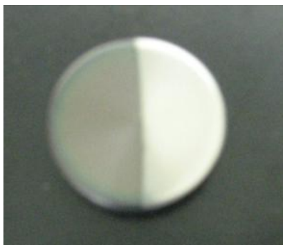
Fig. 9: DLC-coated SKD-11 samples without any interlayers.
