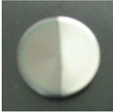
Fig. 4: DLC-coated SKD 11 sample after plasma ashing.
