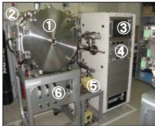
Fig. 1. High-density RF-DC plasma etching system. ① Vacuum chamber, ② RF-generator, ③ Control-panel, ④ RF- and DC-power generator, ⑤ Evacuation units, ⑥ Carrier gas supply.
