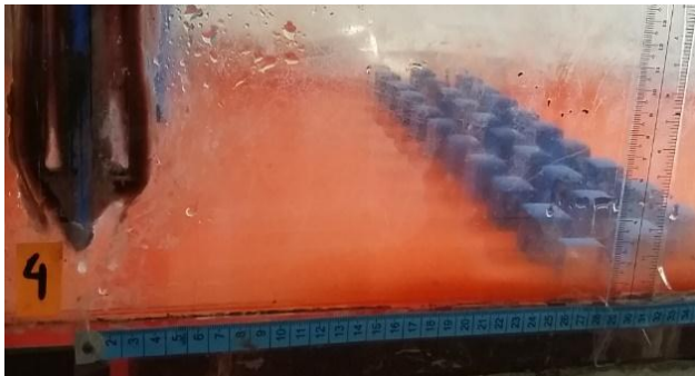
Fig 1. Cubic baffle block configuration in front of sluice gate (source: primary data)
