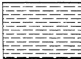
Gambar 8. Aligned discontinuous fibre (Jawed, 2016)
